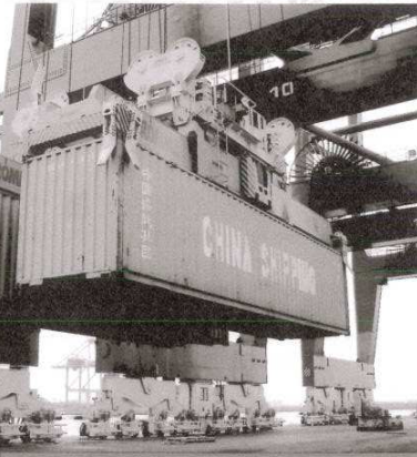
The new cranes at the PSA HNN terminal in the Deurganck Dock are capable of tandem lifts (2 x 40').
